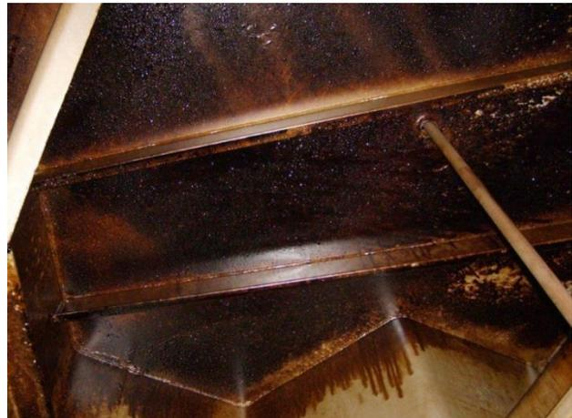
First, each tank needs to be prewashed at 60°C for approximate 1-2 hours. Then the washing water is discharged into a slob tank. Another option is to fill the slob tank with enough seawater to perform recirculation (400 cbm) and use this as the first cleaning step. It often requires two batches to clean the bulk out. Thereafter, those slob tanks must be cleaned in which the cleaning solution is going to be prepared.
